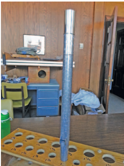
A Swell mixture pipe, returned to its original length
